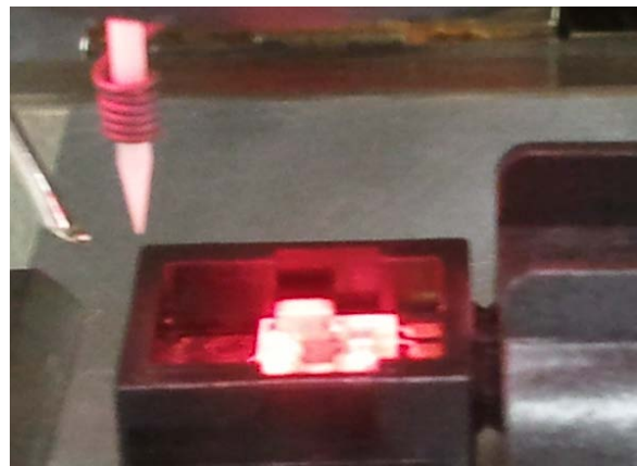
Figure 4 Parts in plastic housing bonded using heated tool.
